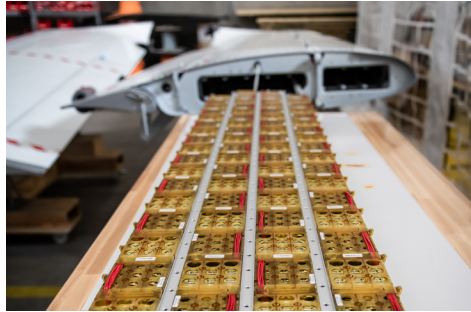
Highly integrated modular energy storage system
